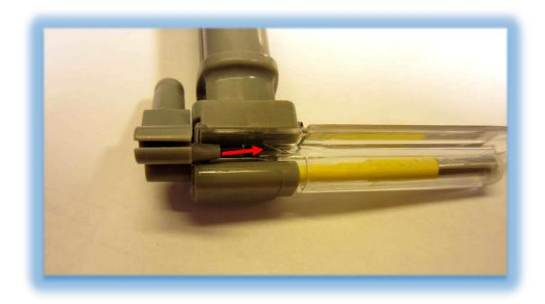
Insert guiding tube in such a way that its rounded tip protrudes from tip of the camera by 3-5 mm but does not protrude from the tip of the blade
